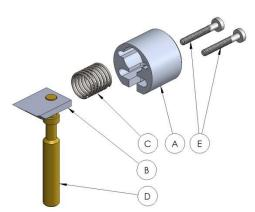
1. Begin by removing the two screws (E) to remove the cutting blade mechanism from the Split Peeler. Be aware that the assembly is under some spring pressure. Make a note of how the blade (B) and lever (D) fit into the cap to help during reassembly.
