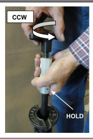
2. While holding the aluminum handle, turn the black T-handle counter-clockwise (CCW) to release the Lockout Plug. Apply slight upward pull to remove the Lockout Plug as soon as it becomes loose.
