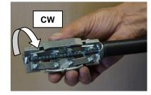
3. While pulling the black T-handle back, unscrew the Lock-out Plug from the Inserter tool by turning it clockwise (CW).
