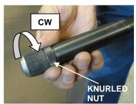
3. While pulling the black T-handle back, unscrew the Lockout Plug from the Inserter tool by turning the knurled nut clockwise (CW).
