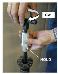
2. While holding the aluminum handle, turn the black T-handle clockwise (CW) to expand the Lockout Plug in the opening. Continue until the Lockout Plug can no longer be moved up or down.
