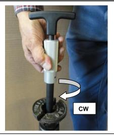
3. Remove the Inserter tool by turning the aluminum handle clockwise (CW) until it comes loose from the Lockout Plug. The Lockout Plug is now installed in the opening.
