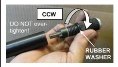
1. While pulling the <u>black</u> T-handle back, insert the Lockout Plug into the Inserter tool as shown and rotate it counter-clock-wise (CCW) until the rubber washer JUST contacts the Inserter tool.
